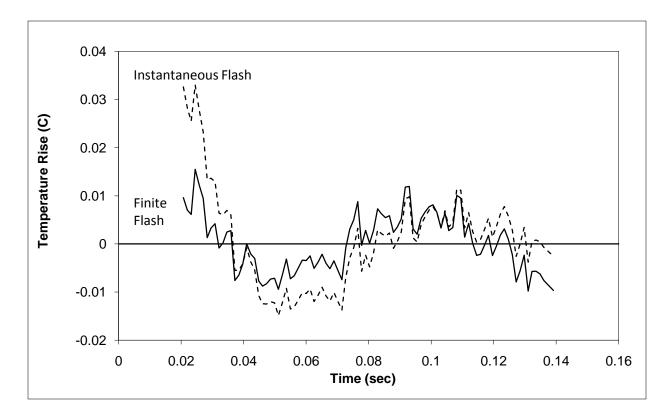
Instantaneous Flash: k = 6.77 W/m-K,  $\sigma$  = 0.01038°C Finite Flash: k = 7.40 W/m-K,  $\sigma$  = 0.00595°C t<sub>1</sub> = -1.91 ms, t<sub>2</sub> = 7.69 ms
