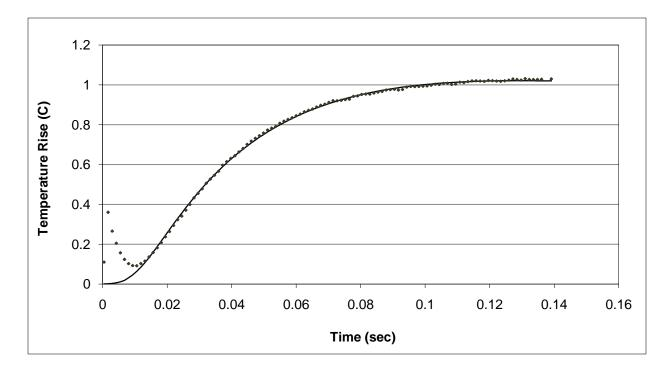
An initial spike in the detector signal from inadequate masking. This mandated a selective use of data.
